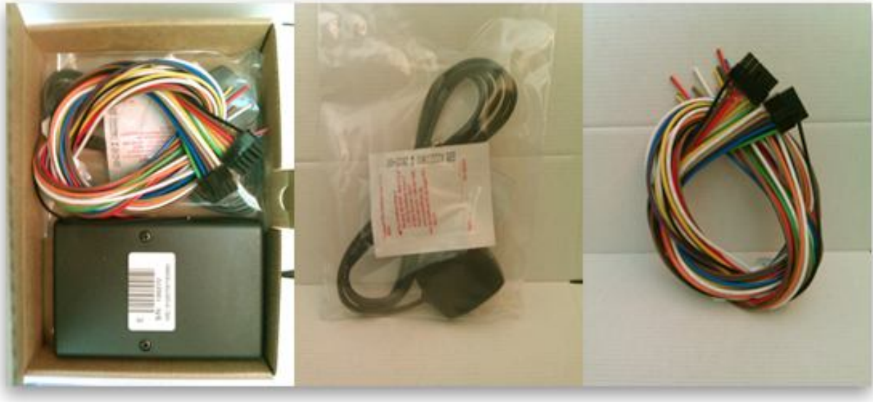
Figure2. FM-Pro3-GLONASS device, power and I/O cables and GPS/GLONASS antenna.
