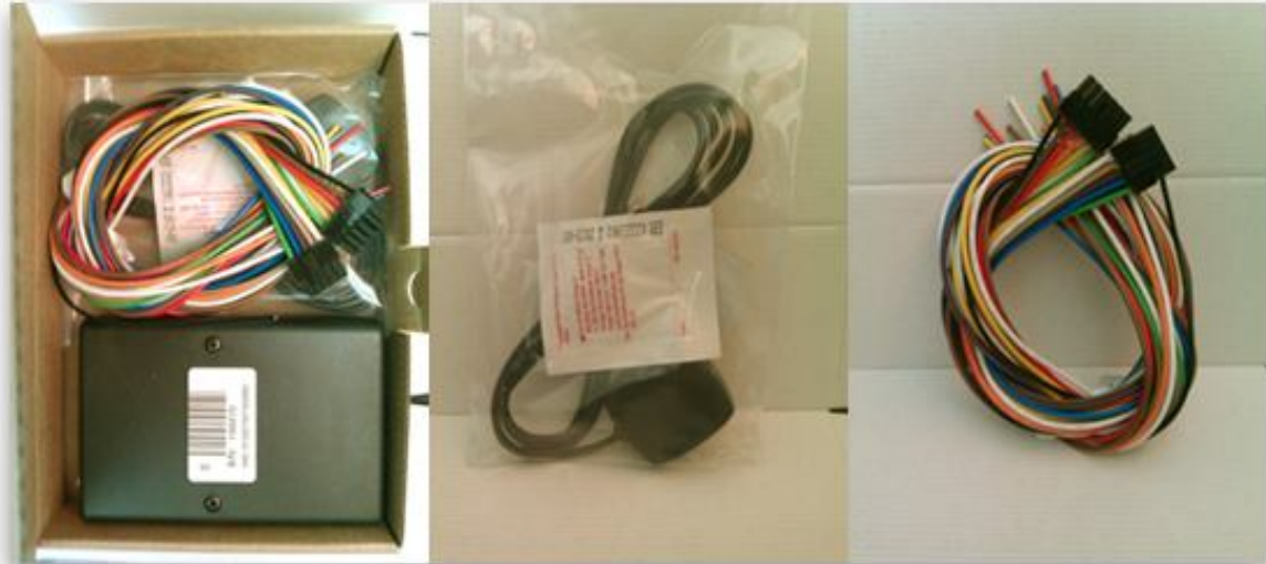
Figure2. FM-Tco3 device, power and I/O cables and GPS antenna.
