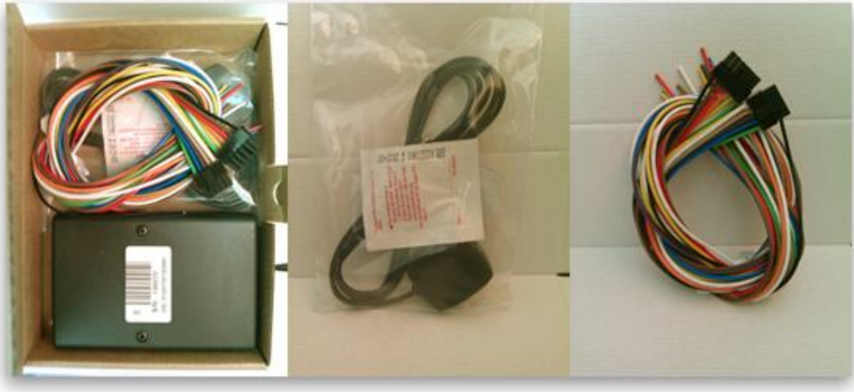
Figure2. FM Pro3 device, power and I/O cables and GPS antenna.
